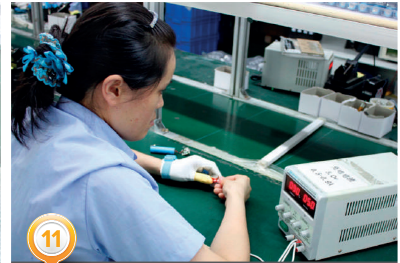
100% manual short circuit test for finished product
