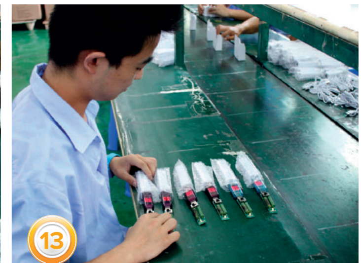
100% load voltage test for finished product
