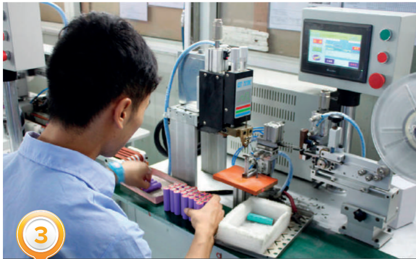
Battery positive pole soldering
