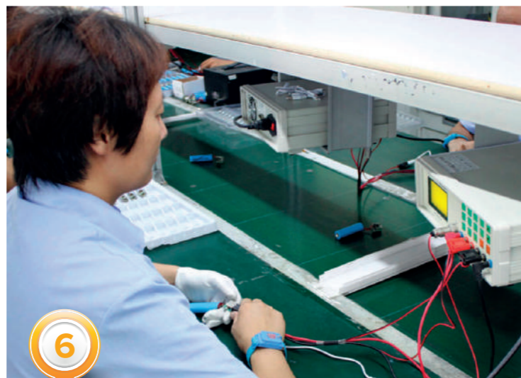
100% over charging and discharging test
