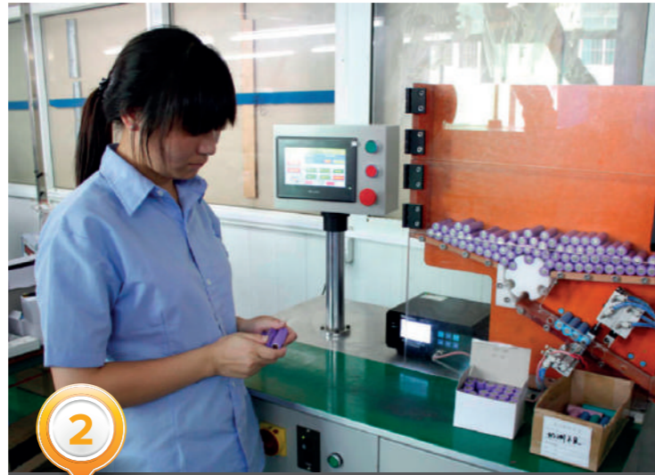
100% battery output voltage test
