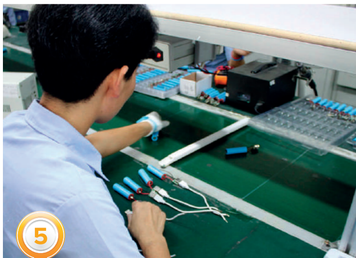
100% manual short circuit test
