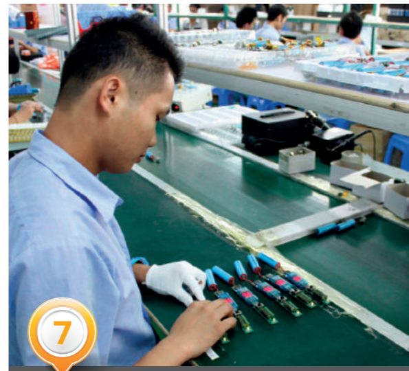
100% load voltage test
